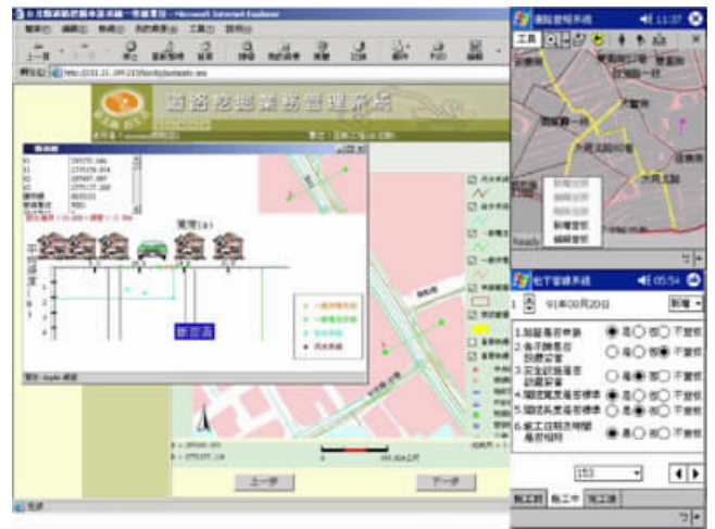
Web-based GIS System for Road Maintenance System
