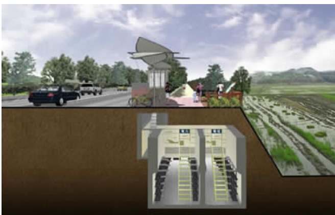
Da-Du Road Common Duct
